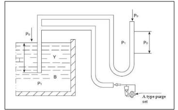
density measure  $\triangle P$  with differential pressure transmitter or pressure meter, then can measure the liquid level h.
